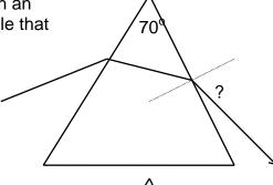
9. Light is incident on an equilateral Lucite prism (n = 1.5) at an angle of 35°. Calculate the angle that the light leaves the prism. (66°)
