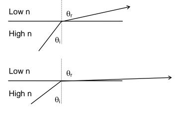
At the angle of incidence called the **critical angle**  $(\theta_c)$  the angle of refraction =  $90^\circ$ .
