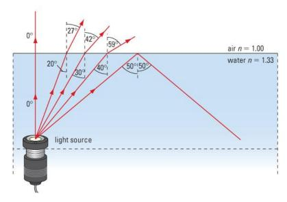
The properties of internal reflection are used in fibre optic technologies and in optical instruments like cameras, microscopes, binoculars, etc.
